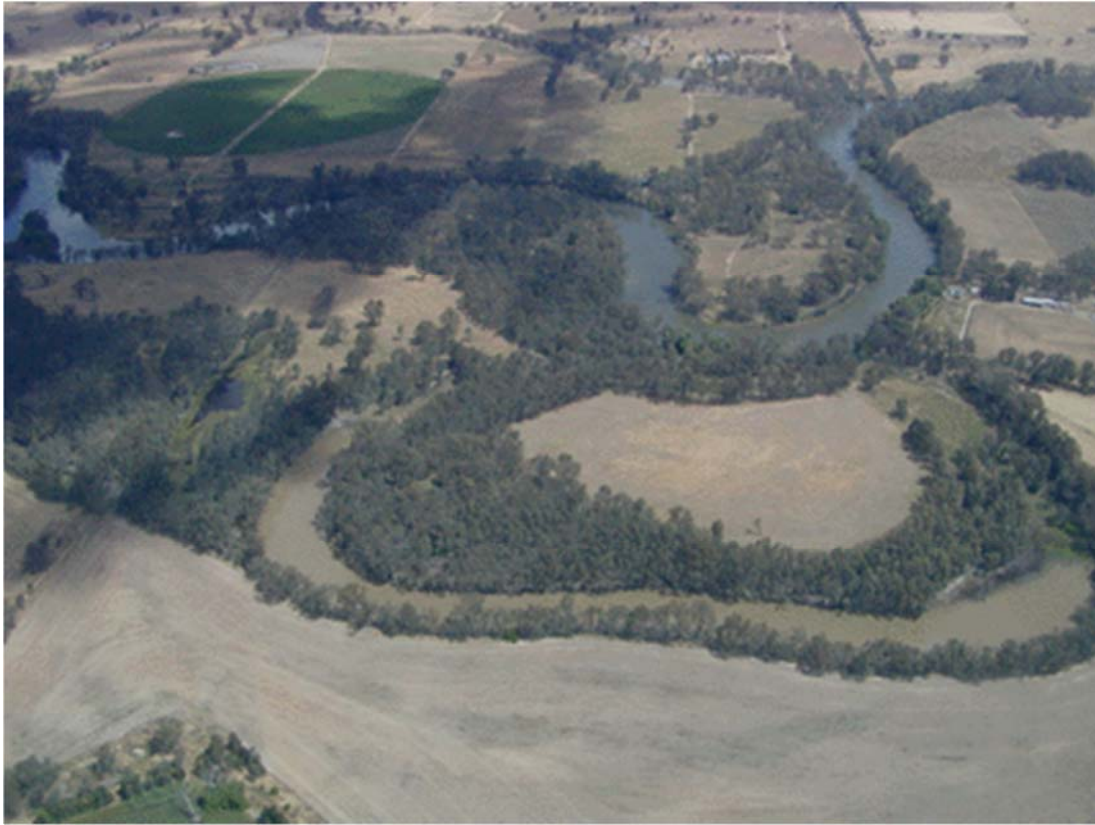
The tree-lined but abandoned channel in the lower part of the photograph shows the former course of the Murrumbidgee river (SE Australia) at this meander bend.
