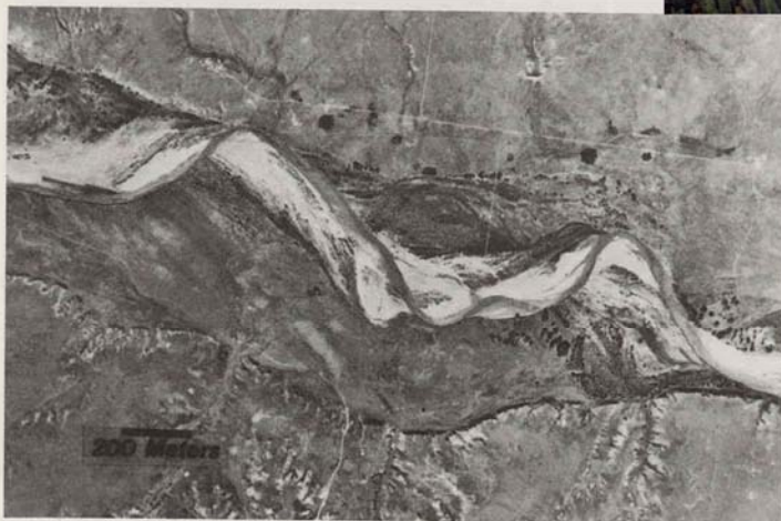
Figure 2.8 Sinuous braided river: North Canadian River near Guymon, Oklahoma at low stage. Point bars are marked by braided pattern. (Courtesy of J. S. Brice.)
