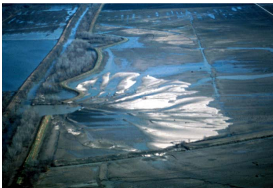
Crevasse splay sand from levee break at Bryants Creek MO crossing floodplain of upper Mississippi River near mile 260. Photo by R.H. Meade, USGS
