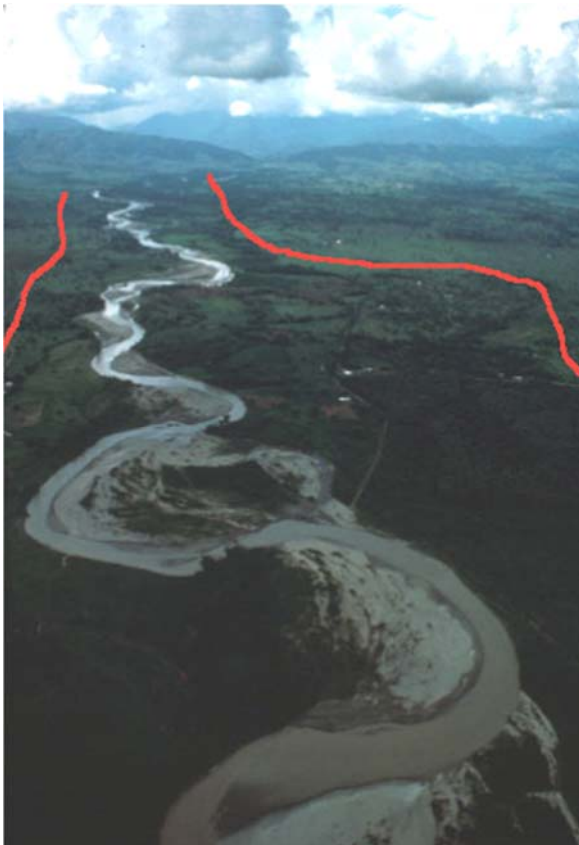
Río Socopo flowing off eastern slope of Venezuelan Andes. View is up river (towards WNW). October 24, 1984. Note point bars along inner bends. The channel belt is defined as the region between the red lines within which the active channel tends to meander. Photo from R.H. Meade, USGS
