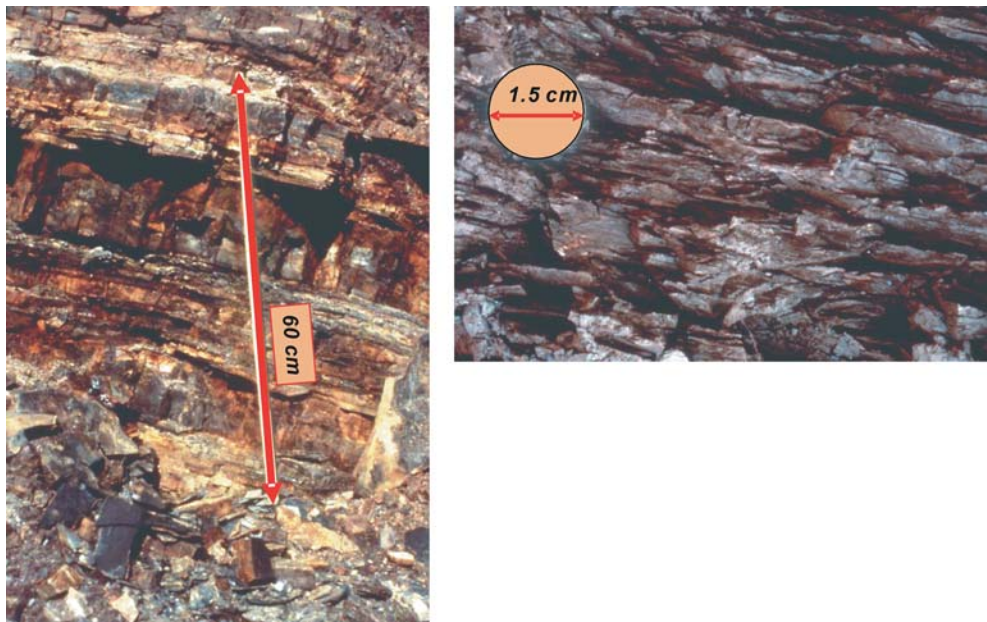
Fig. 12 The Brindisi di Montagna highly-fissured clay shale (from Picarelli et al. 1998): (a) parent flysch formation; (b) fine grained component
