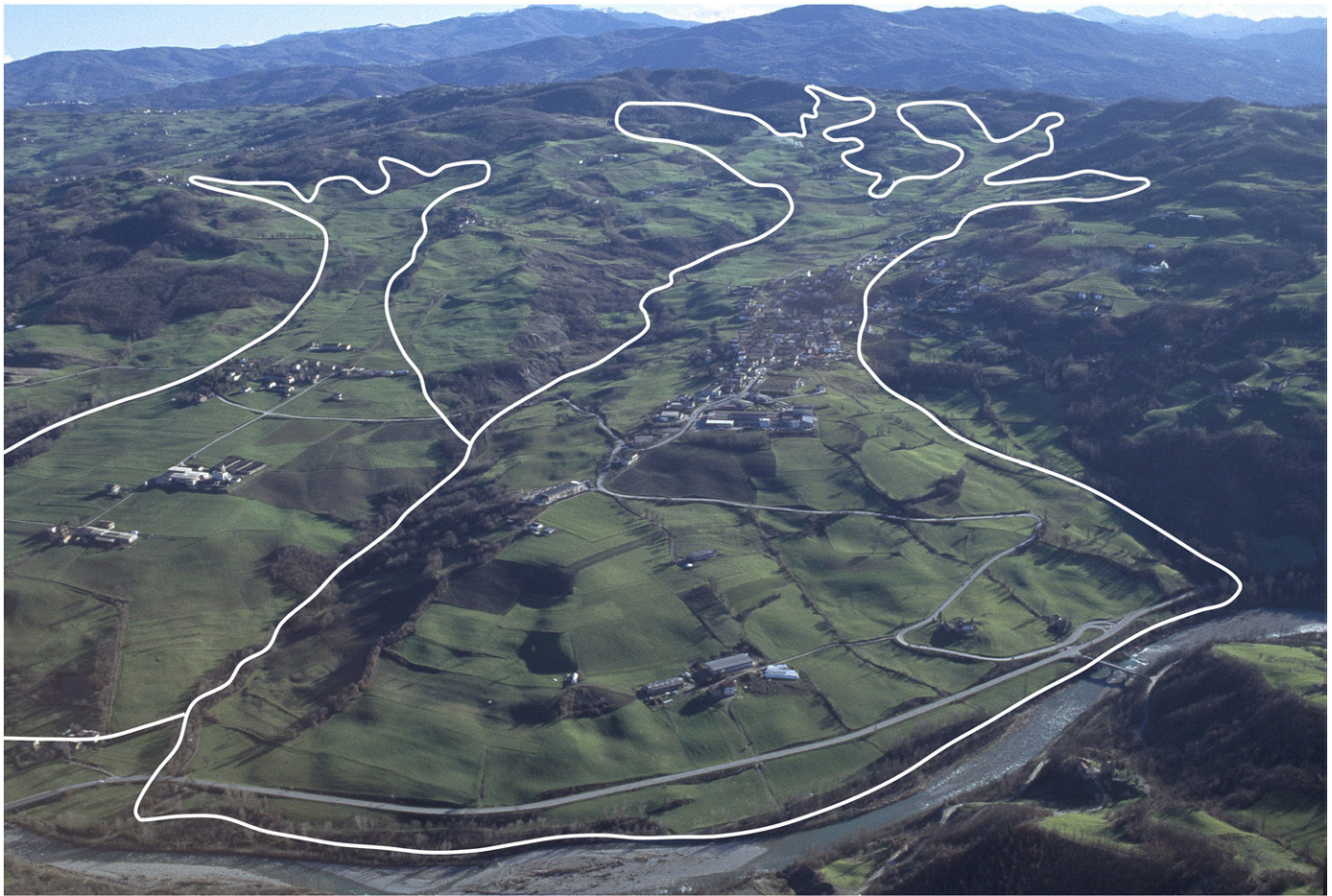
Fig. 3. The Cavola (right) and Oca (left) landslides. The 4.2 km long Cavola landslide is considered inactive since 1960, but it still shows movements at instrumental scale. See also Fig. 5. Photo by G. Bertolini (2005).
