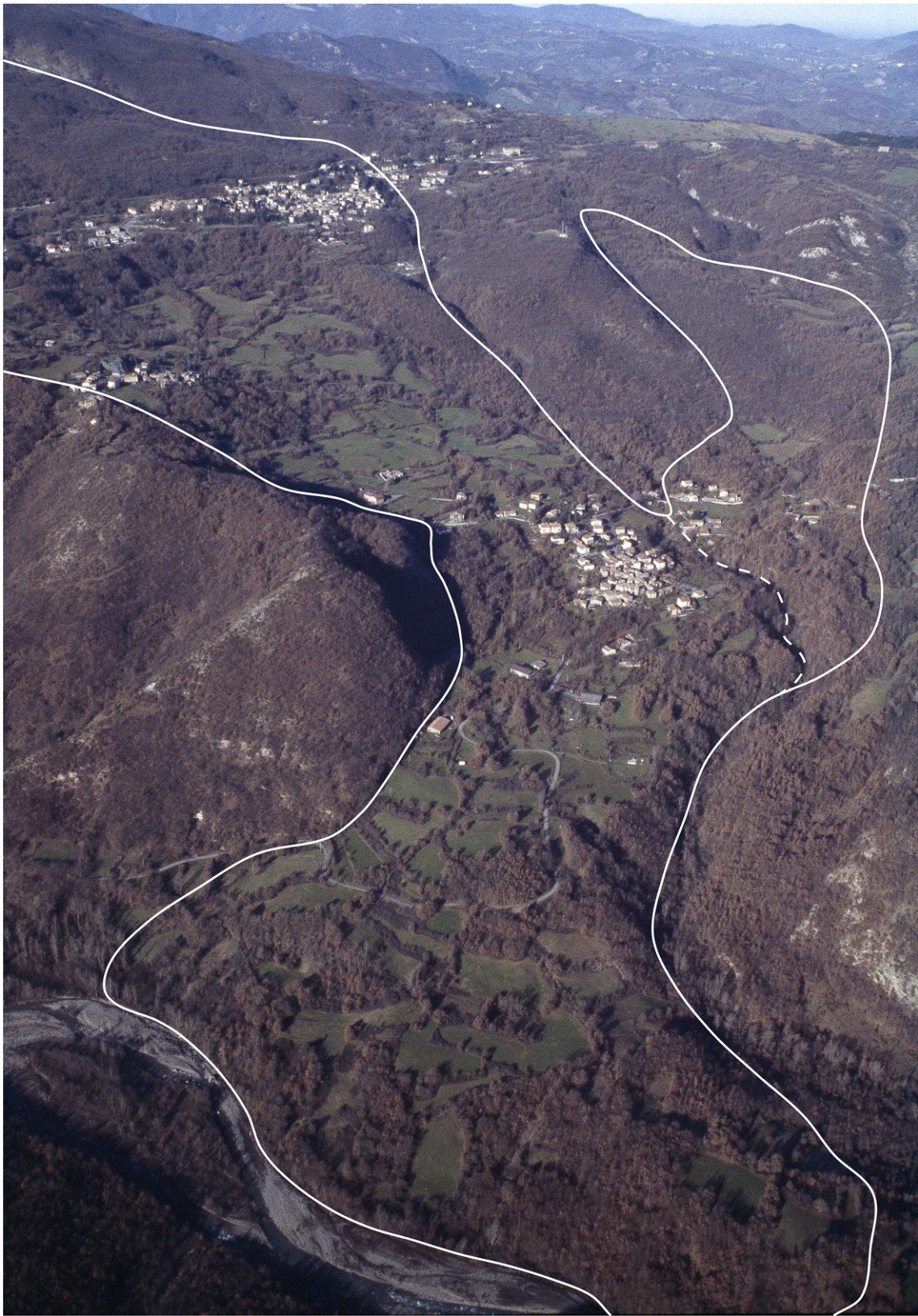
Fig. 8. The large, dormant Cervarezza landslide. Photo by G. Bertolini (2005).
