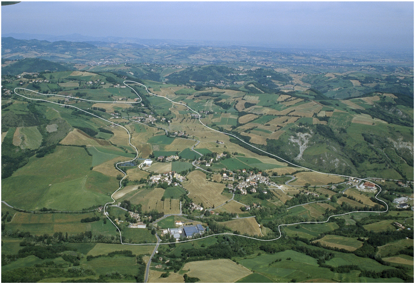
Fig. 15. The Provazzano landslide in Province of Parma symbolises the problem of risk assessment and management in ancient, dormant earth flows. Five villages and several factories lie “undisturbed” on it. Villages have grown, during the last centuries and decades, almost only on the landslide that is the smoother area and seems the most reliable site of the slope. Photo by G. Bertolini (2006).
