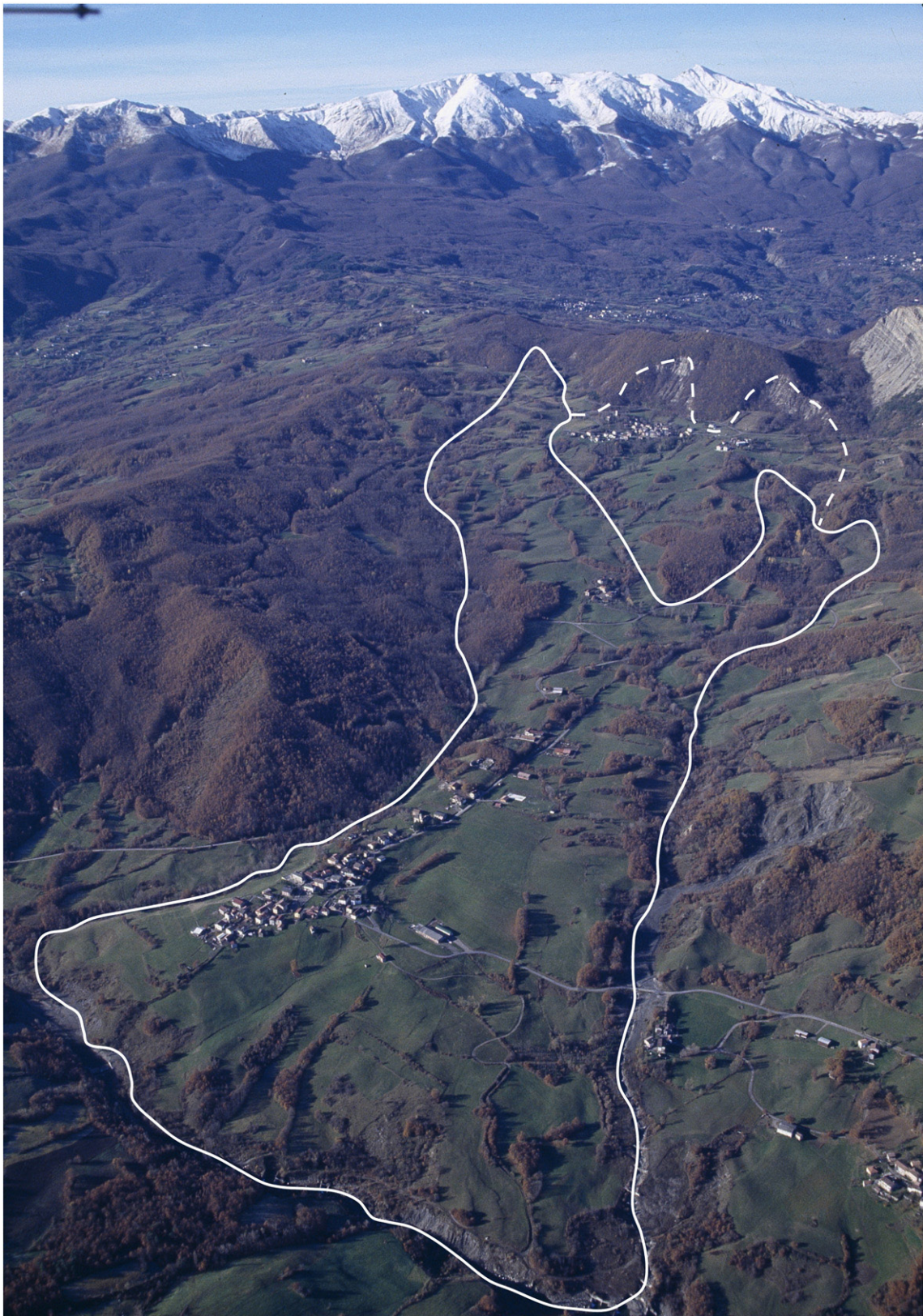
Fig. 2. The Large Morsiano Landslide. Despite its age (a wood sample found inside it dates back to 13,500 Cal. years B.P) the landslide is still active in several portions, threatening and damaging the village. According to historical records, reactivations occurred in 1631 (partial), 1651 (total), 1880 and 1959 (partial). Photo by G. Bertolini (2007).
