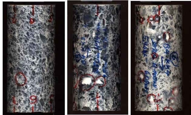
Fig. 2: Salt concrete sample before testing
