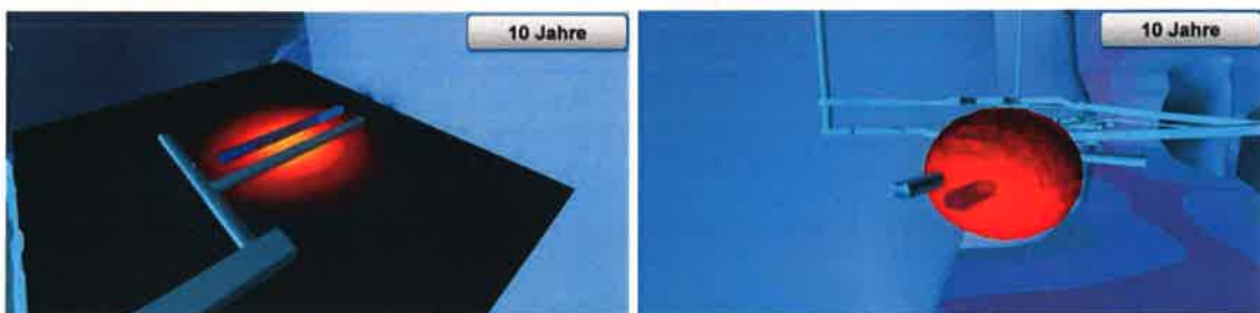
Figure 1(c): Visualisation of the temperature field around two drifts heated by POLLUX casks ( left : horizontal section, right : 3D evolution)
