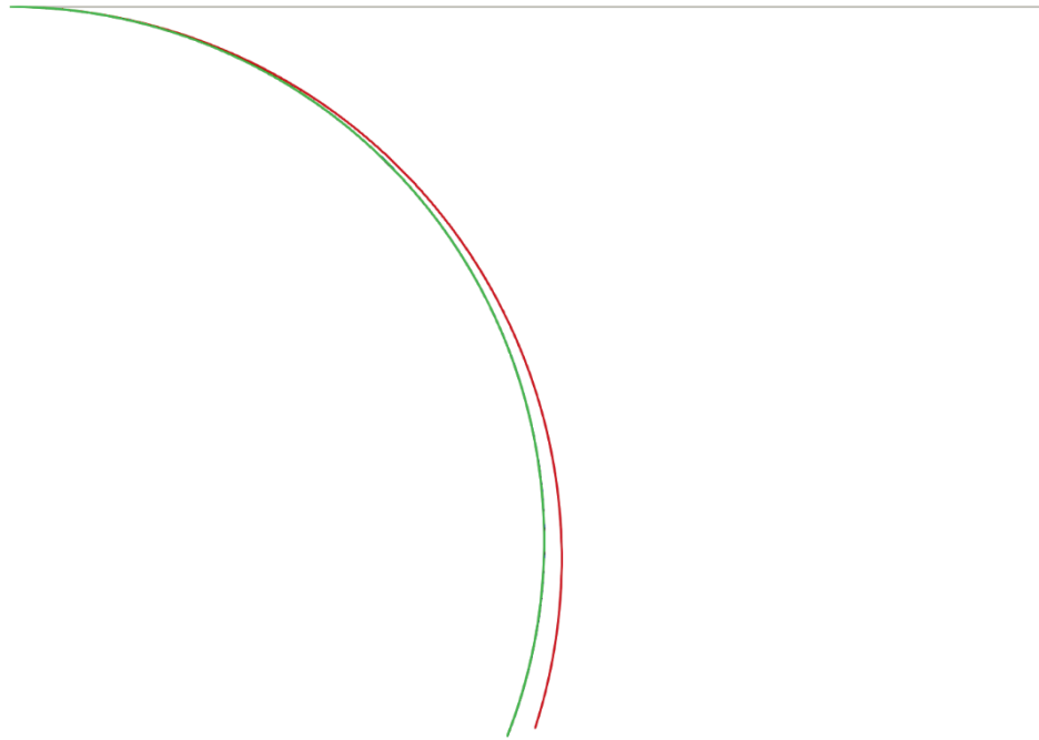
FIGURE 11 | Electrically induced bending beam. Deformation of the beam for AR = 500 using the finest mesh with N = 2048 FEs along the length. up\phi Q1 (red), up\phi Q2 (blue), upS'\phi Q1 (green), and upS'\phi Q2 (black).
