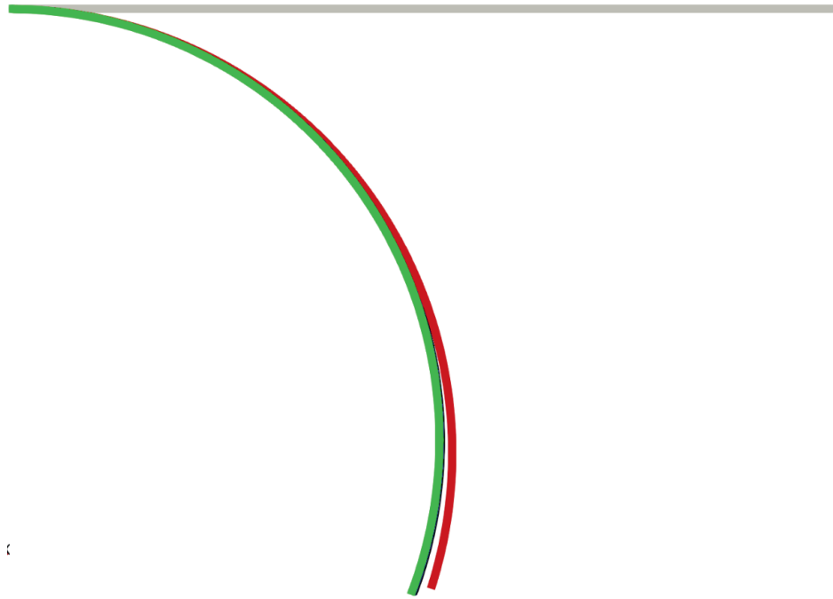
FIGURE 9 | Electrically induced bending beam. Deformation of the beam for AR = 100 , using the finest mesh with N = 2,048 FEs along the length. up\phi Q1 (red), up\phi Q2 (blue), upS'\phi Q1 (green), and upS'\phi Q2 (black).
