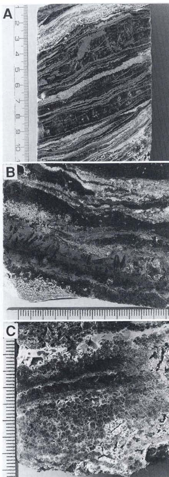
FIG. 9.—Polyhalite facies: (A) laminated polyhalite (scale in cm), (B) polyhalite pseudomorphs after glauberite in laminated polyhalite facies (scale in mm), and (C) spherulites of polyhalite with carbonate matrix (scale in mm).
