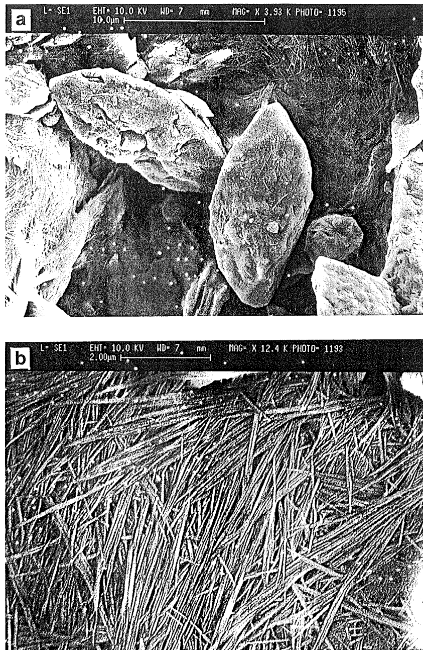
Fig. 4. Scanning electron micrographs of palygorskite from a marginal saline lake sample (AU section). (a) Mats and scattered fibres coating lenticular gypsum. (b) Close view of palygorskite mats.
