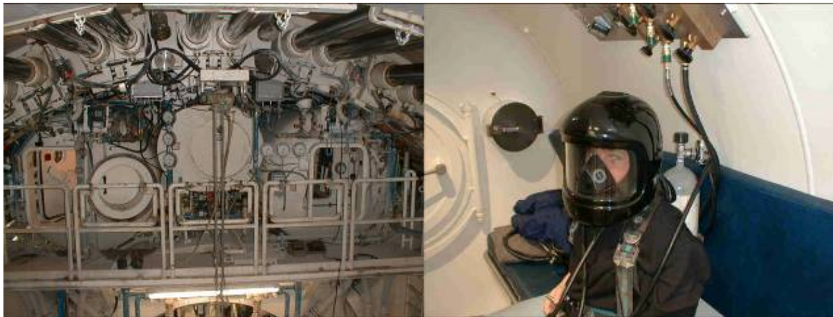
Figure 13: Lock with additional transport flange, diver with helmet for Trimix-gas (Thewes, 2007b).
