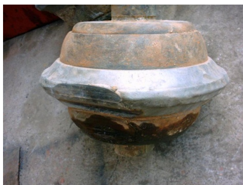
Figure 25: Damaged disc cutter that has run flat (Thewes, 2004).
