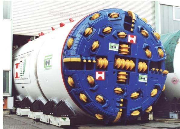
Figure 15: EPB-shield for an application in a mixed-face situation with soil and rock (Thewes, 2004).
