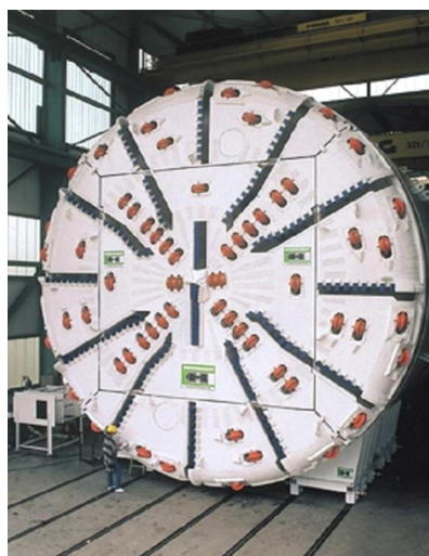
Figure 16: Slurry-shield for an application in a mixed-face situation with soil and rock (Thewes, 2004).
